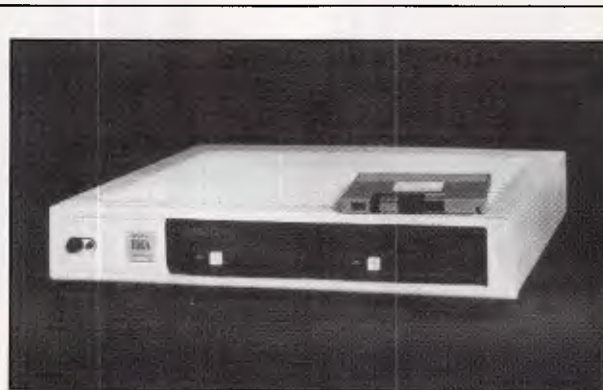
This is a removable hard disk device from IDEAssociates, a sizeable US operation which has just set up offices in Australia. Each of the two disks contains 10Mb and the unit has a 'zero' footprint, meaning it sits between the top of your PC and the monitor.
